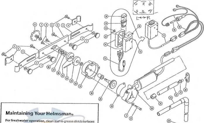
For freshwater operation, clean and re-grease clutch surfaces and needle bearing after every 50 hours or so of use.
